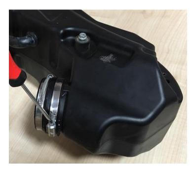
TIP! Open the OEM airbox from top, remove the filter and put one hand in to better push out the intake and use your second hand to pull it out... you have to queeze it before the end to get it out! Dont worry – it is rubber and it has the shape memmory.
