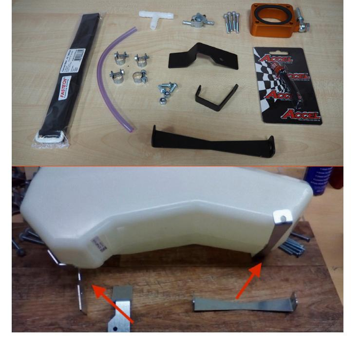
Start mounting the small airbox into the bike.
