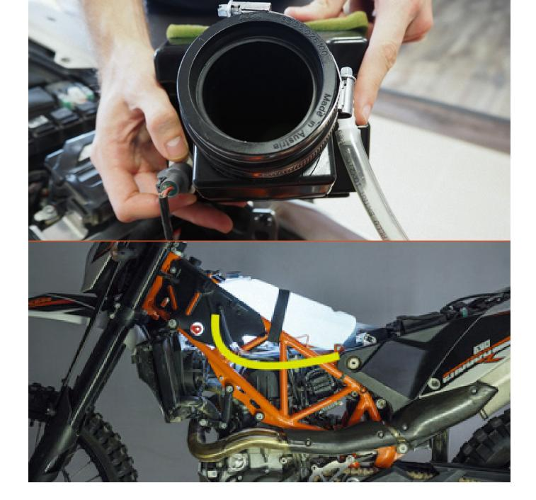
— Before you insert the "small airbox" into the bike, make sure you connect the vent tube and electrical connector to the heat sensor!
