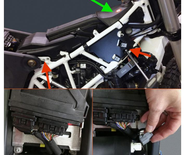
Remove the seat, side panels and take out the airbox.
