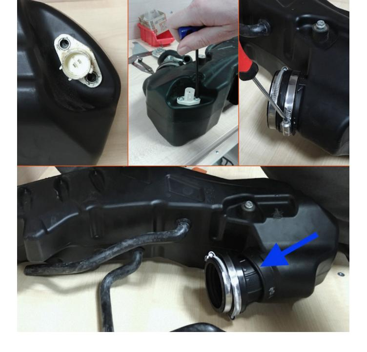
Remove the intake and heat sensor.
