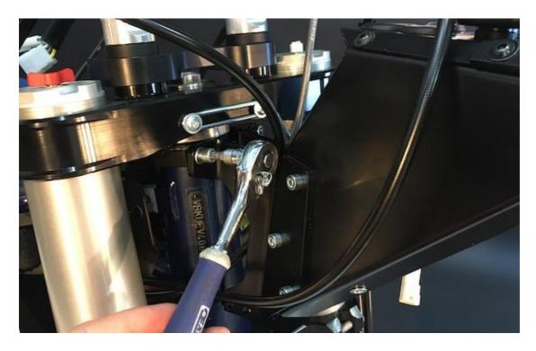
d/ Now lift the tower a bit to be able to pull inside (start from the bottom) the harness and cables as in the picture.
