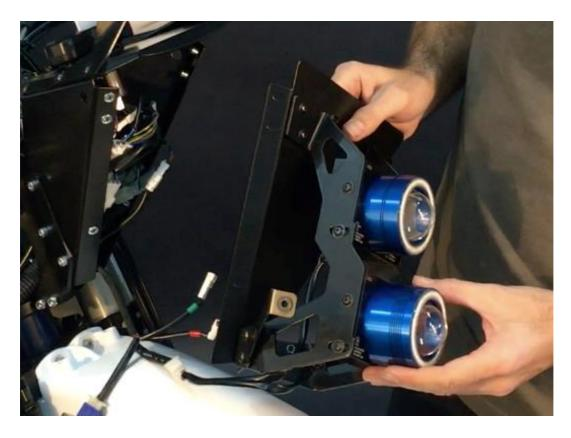
c/ Before you bolt on the holder don't forget to connect the headlight connector and make sure the turn signal connectors could be reached from the bottom. Also test the headlight's low and high beams.
