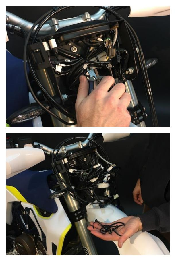
b/ First mark the indicator cables (what is what) before you disconnect them. it will make assembly easier © Next, remove the indicators from the dash panel.
