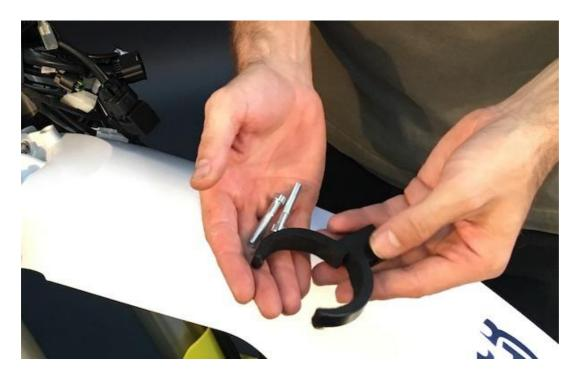
f/ Lift the tower a bit (you can use your shoulder) and with your hands insert from the bottom both clamps at the same time and insert the bolts. It needs a good alignment of the holes to be able to push the bolts through. IMPORTANT! Make sure you do not squeeze any of the cables! All the cables must be above the lower clamp.
