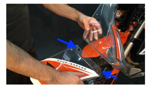
d/ Insert the M5 rubber nuts into the windshield – but leave the middle hole free.
