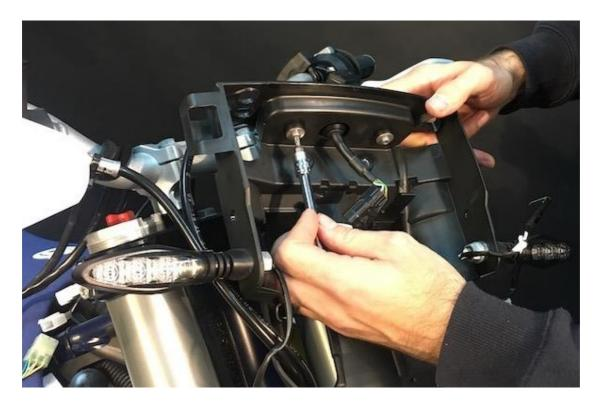
e/ Coming from left side and turning the handlebars to the right, loose the M5 bolt and bent the black plastic cover. You will see three connectors from the throttle. Disconnect them.
