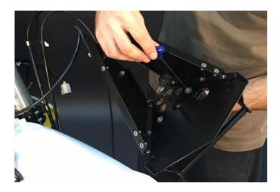
c/ b/ Also insert the three large supplied grommets into three large holes and insert the controls (not yet iinserted n this picture). And install in the 12V USB outlet.
