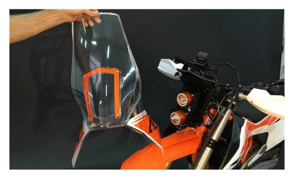
g/ Place the fairing o the tower and bolt on four holders with M5x16
