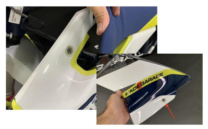
i/ Now put on the seat and lock it into the R/G panels. This will fix the fairing panels to the motorbike.
