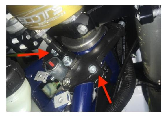
c/ Use M6x20 bolts and washers to bolt on the tower to the top clamps. Don't tighten at this stage!
