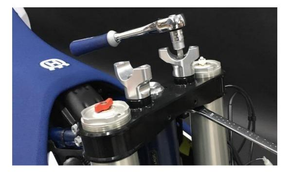
b/ Take the R/G adapter and M10 bolt – don't forget to loc-tite! and bolt on. It is a bit tricky to tighten it parallel for precise fit of the handlebars, so take your time! Perfect alignment is crucial.
