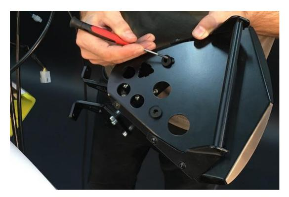
b/ Mount the speedo with the original screws.
