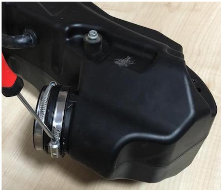
TIP! Open the OEM airbox from top, remove the filter and put one hand in to better push out the intake and use your second hand to pull it out... you have to squeeze it before the end to get it out! Dont worry – it is rubber and it has the shape memmory.
