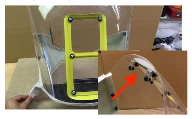
10b/ Mount first together the fairing side panels and windscreen only on four M5x16 bolts and ruber nuts.
