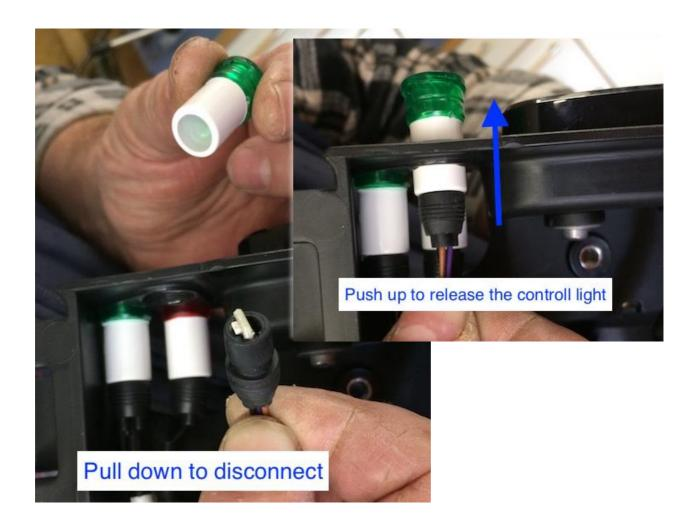
4c/ take very small screw driver or knife and press the three secure pins and push the ABS button upwards to get it out
