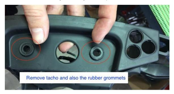
4b/ disconnect the control lights as on the pix and push the controls upwards to get them out and keep them for later!
