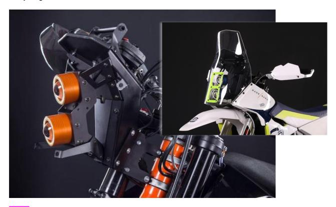
NOTE: It is highly recomned you install everything finger tight first to ensure proper fitment and alignment, then go back and tighten everyhing up. On botls that DO NOT have a nylon-intsert lock nut, I reccomend using blue loctite on the bolt threads.
