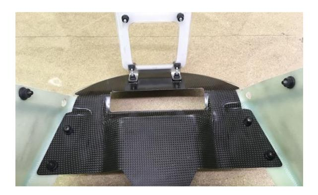
11a/ Insert the rubber nuts into the four fairing holders as on the pix.
