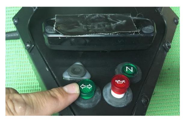
5c/ Insert the ABS button and secure it from bottom side with supplied rubber triangle grommet as on the pix.
