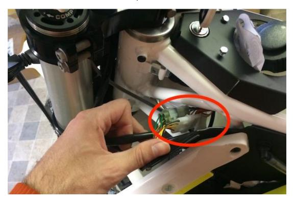
3b/ Next you have to completely remove away the black plastic part. To be able to do so, you have to cut it in left down corner by sharp knife or blade and take out the cables.
