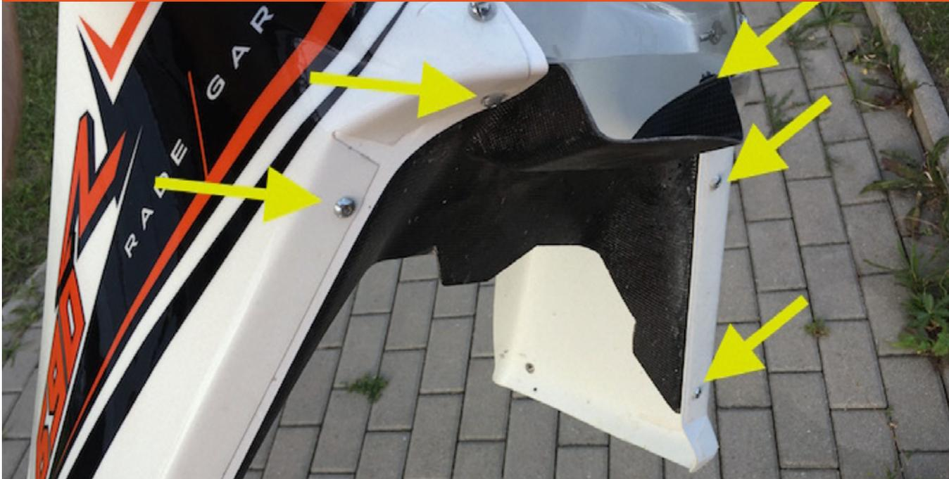
— After mount the connected fairing panels to the windscreen and to the OEM side panels.
