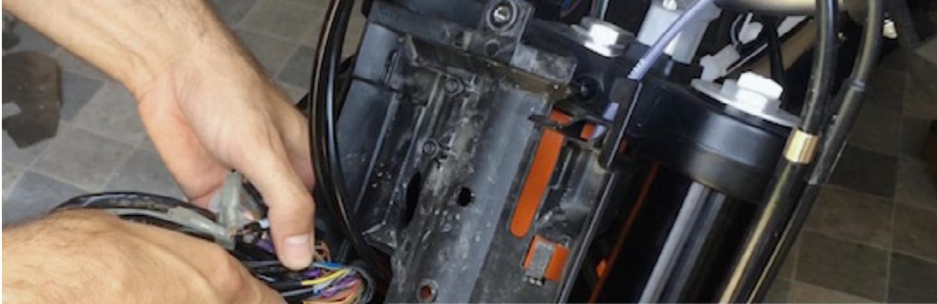
To get out the cables, cut with a knife the plastic part here
