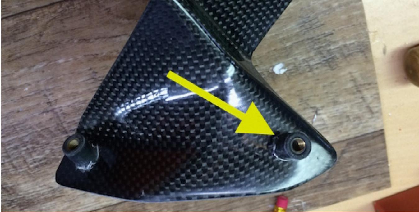
— Now insert the carbon connection part between the side fairings. To connect the carbon connection part to the fairing panels use the 4× rubber nuts and M5×16 bolts.
