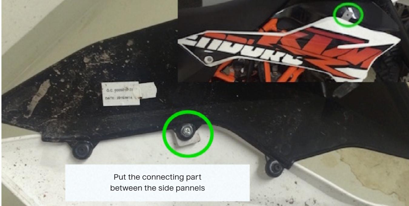
Put the connecting part between the side panels
