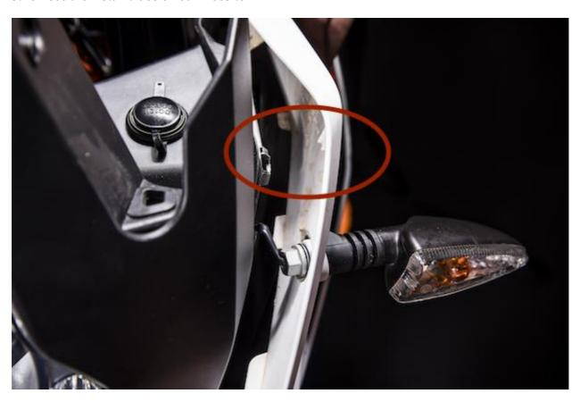
c/ Next remove the upper two bolts holding the headlight.
