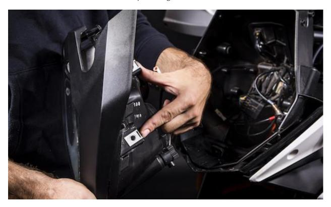
b/ Assemble the LED headlights. The high beam with shorter tube goes to the upper position and the low beam with longer tube goes below. Use the M5x16 black bolts. Bolt on the orange resistors with M4 bolts. Use the rubber nuts for the upper carbon mask holders and supplied M5 nut inserts for the bottom mask holders (they are not pictured).
