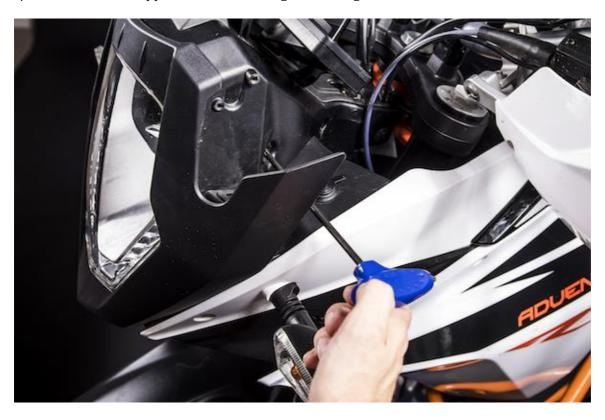
$\mbox{d}/\mbox{ To access the bottom bolt, you have to carefully bent the side panel and remove the OEM bolt$
