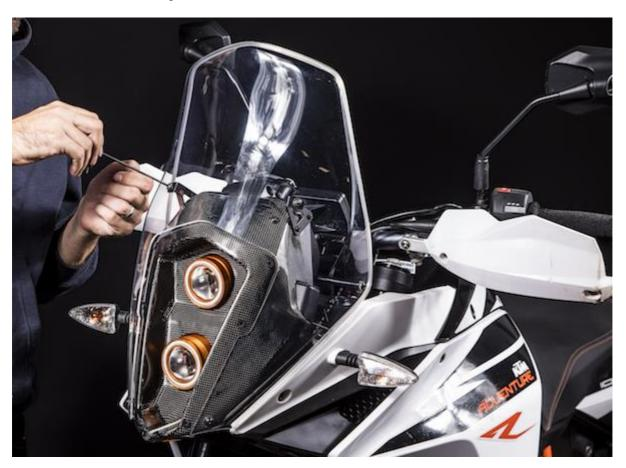
b/ When mounting the lower bolts use the rubber distance washers in between the carbon mask and the windscreen. Before you insert the bolts align (using a guide e.g. small screw-driver) the nut insert with the hole in the carbon mask.
