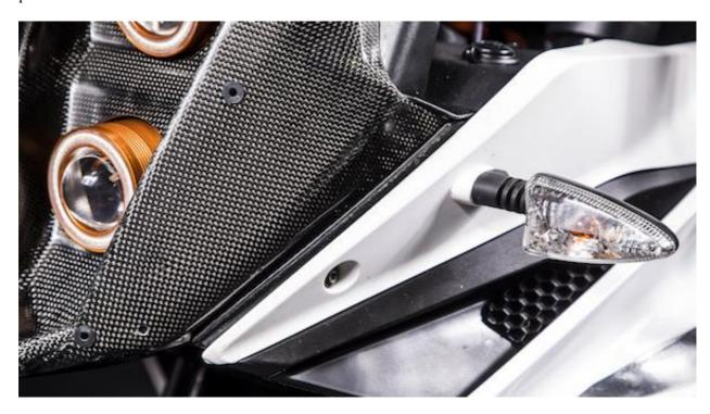
c/ Bolt on the mask to the upper bracket with M5x16 bolts and use the plastic washers. Also mount the top windscreen holders with the OEM screws.
