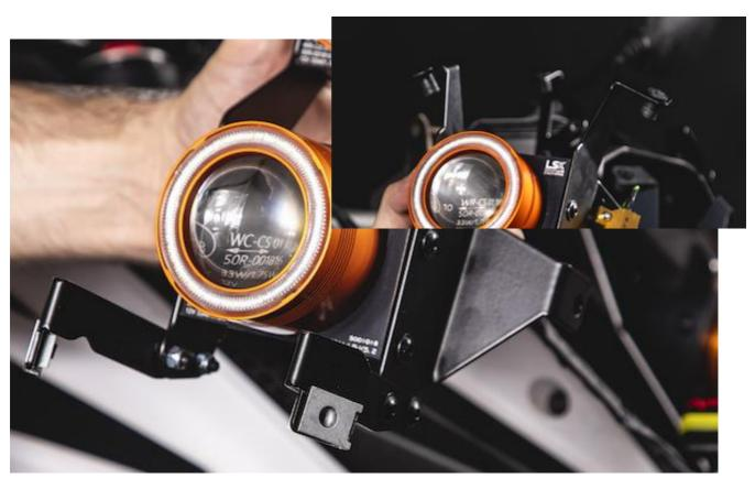
c/ Tip for you! Before you connect the LED unit, you have good opportunity to connect your GPS cable, heat grips cable and other accessories, because the OEM spare power source is now easily accessible.
