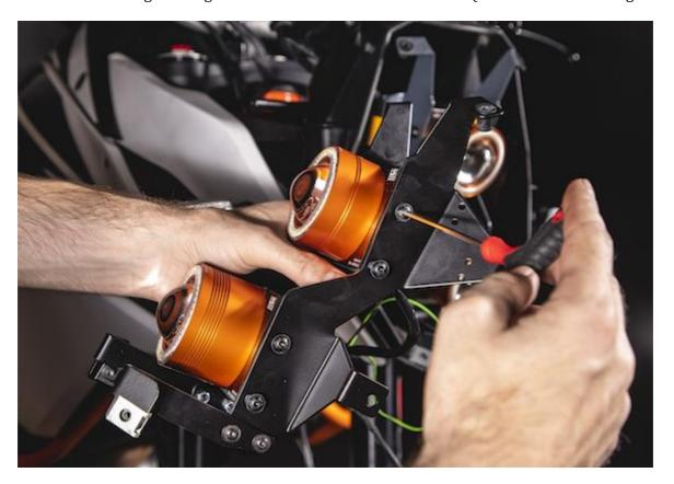
c/ Bolt on the orange resistors with M4 bolts and nuts.
