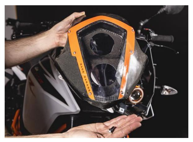
b/ When inserting the carbon mask make sure it is placed under the OEM black plastic rim as in the picture.
