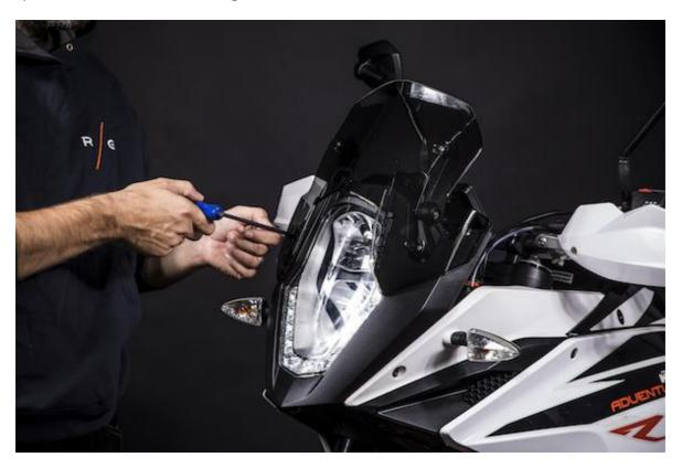
b/ Lift up the OEM screen holders and remove the plastic holder bolts as in the picture. Remove also the metal plates and keep the OEM screws for later.
