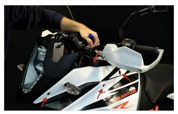
b/ Hold the turn signal and CAREULLY lift up the white panel – there is a plastic hook on the back side. You must remove the white panel in order to access the bolt holding the OEM headlight. If you are not sure – see the install video on our website.
