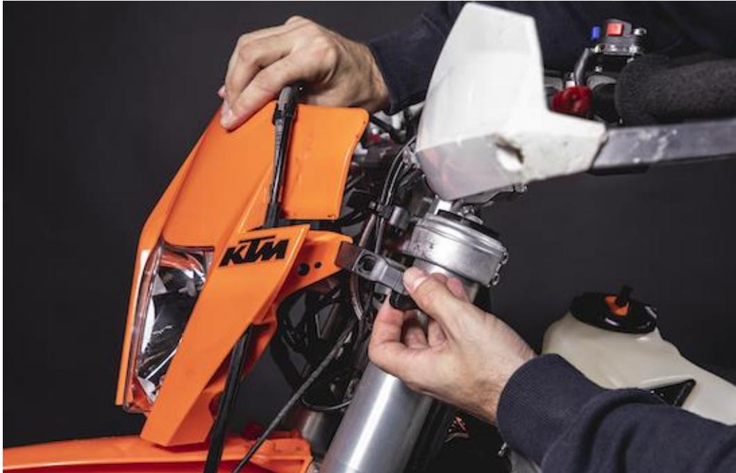
b/ Cut carefully the zip ties and remove the black plastic holder of the electric cables. Also remove the speedo holder and disconnect the speedo.
