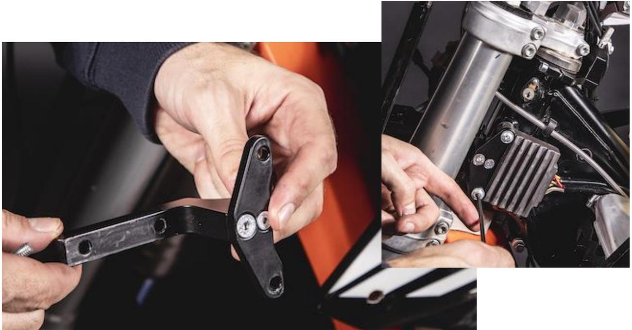
b/ Remove the tie holding the cables. Use pliers and drag it out. Next take out the fuel overflow tube and screw out the plastic L-connection from the frame.
