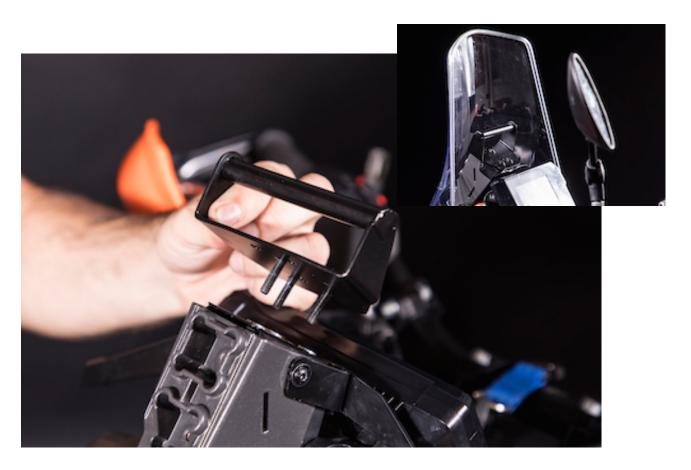
e/ Take the supplied metal hooks. First put in the rubber nuts and then insert one metal hook on each side in place the of the original OEM spoilers.
