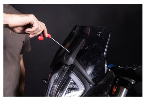
b/ Behind the spoilers are bolts, one on each side. Remove them. Then carefully lift each spoiler up. They have plastic hooks locked in the plastic tower – don't use force! (RISK OF BRAKING)
