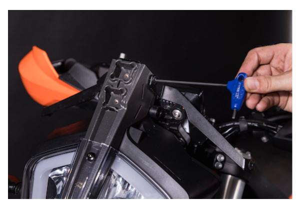
d/ Use the 3 supplied longer M5 bolts to attach the GPS bracket. It can be situated closer or further from the windshield. We recommend the orientation CLOSER to the windshield.
