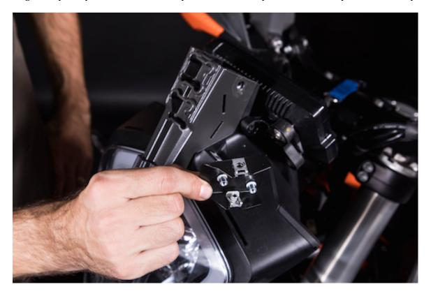
c/ Replace bolt in the main bracket with the supplied M5x16 bolts. Also insert the rubber nuts into both sides of the main bracket.
