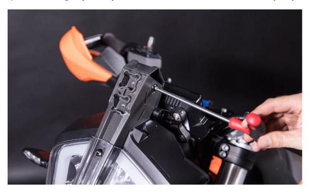
b/ Take the supplied metal plate with the 3 rivet nuts. Then remove the threat inserts from the original cap and put them in the metal plate. When done, place this assembly instead of the plastic cap.
