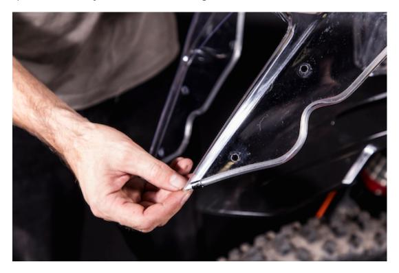
b/ Mount the windscreen with the M5x16 bolts. To avoid the metal holders scratching the windshield place in between the windscreen and the metal holder the supplied rubber washers. It means the rubber washer goes under the windscreen and the white plastic goes under the bolt's head.
