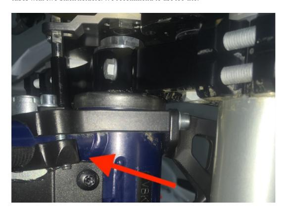
b/ bolt on the PIN holder with short M6 bolts. Also loc-tite
