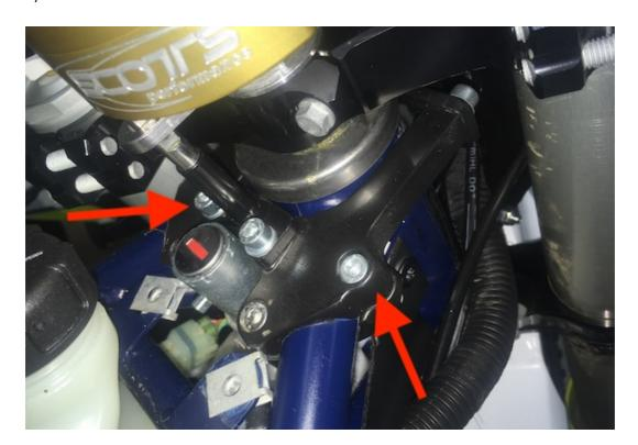
$c/\,\text{Use M6x20 bolts and washers to bolt on the tower to the top clamps.}\,Don't\,tighten\,at\,this\,stage!$
