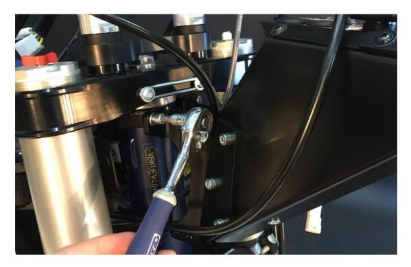
d/ Now lift the tower a bit to be able to pull inside (start from the bottom) the harness and cables as in the picture.
