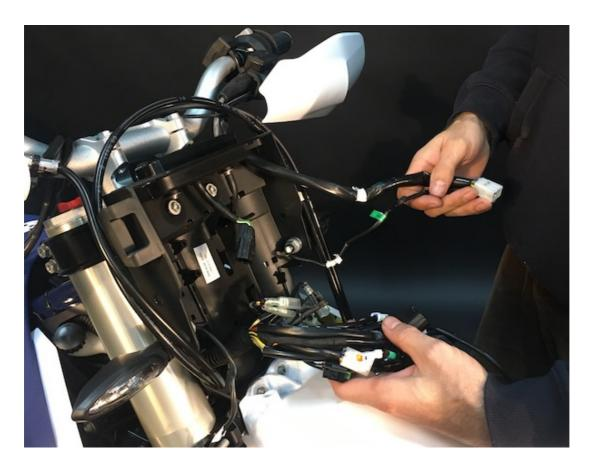
g/To remove the black mask holder, you have cut the plastics with a sharp knife or a saw. This will allow you to remove the mask holder from the brake/ABS hose.
