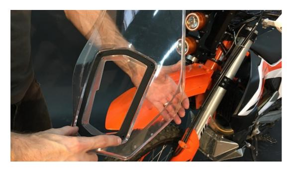
b/ Install the orange/yellow sticker on the headlights cover and bolt on with M4x16 bolts using the plastics washers.
