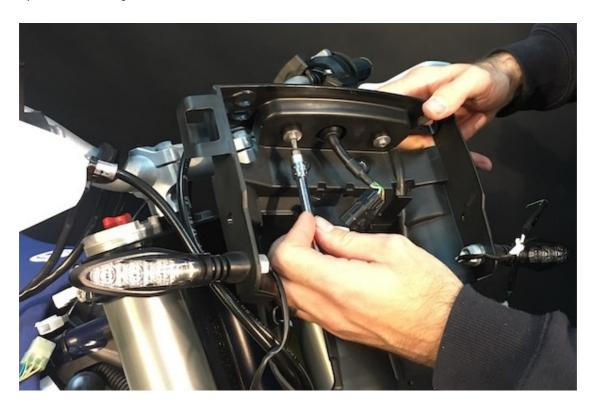
e/ Coming from left side and turning the handlebars to the right, loose the M5 bolt and bent the black plastic cover. You will see three connectors from the throttle. Disconnect them.
