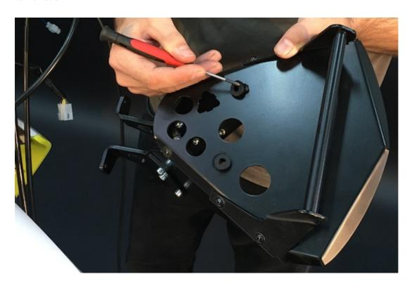
b/ Mount the speedo with the original screws.
