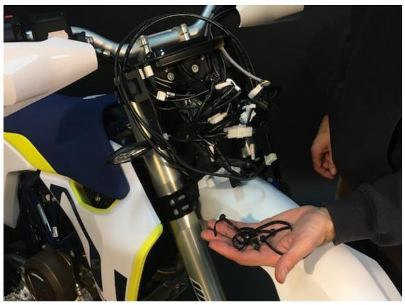
b/ First mark the indicator cables (what is what) before you disconnect them. it will make assembly easier © Next, remove the indicators from the dash panel.
