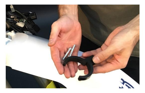
f/ Lift the tower a bit (you can use your shoulder) and with your hands insert from the bottom both clamps at the same time and insert the bolts. It needs a good alignment of the holes to be able to push the bolts through. IMPORTANT! Make sure you do not squeeze any of the cables! All the cables must be above the lower clamp.
