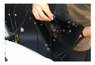
c/b/Also insert the three large supplied grommets into three large holes and insert the controls (not yet iinserted n this picture). And install in the 12V USB outlet.
