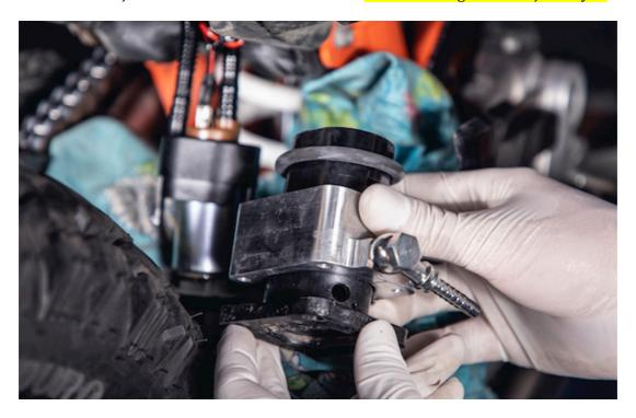
d/Bolt on the spacer with supplied bolts. Be careful to don't destroy the threads in your tank. When it is done, put back the mud guard.
