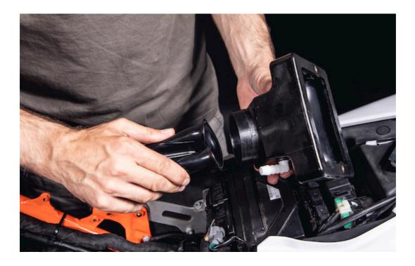
$\ensuremath{\text{c}}/$  Attach the pink vent tube and then fit the small airbox back on the engine suction neck.
