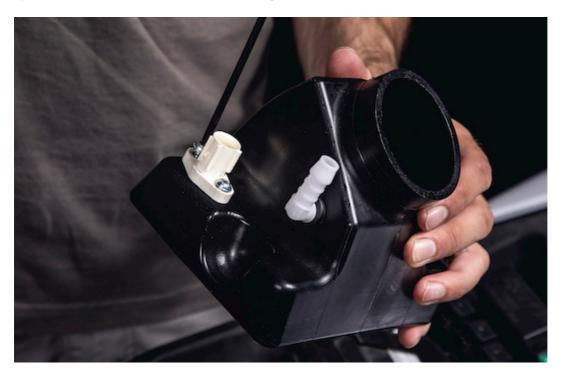
$\ensuremath{\text{b}}/\ensuremath{\text{Squeeze}}$  the original flange as in the picture and insert it into the small air box.
