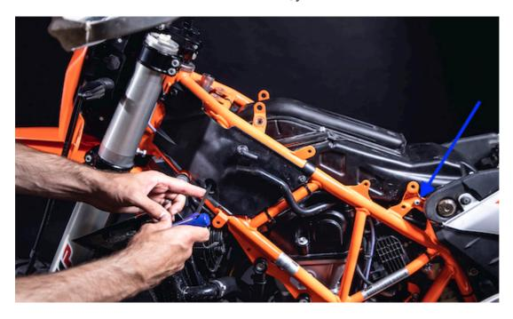
c/ On the left side of the bike... loose the sleeve holding the air box flange. Note, there are two sleeves – loose the one closer to the engine! Then take again big flathead screwdriver and push the flange out of the engine suction neck and remove the air box.
