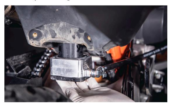
e/ Use supplied bolt and spacer to mount the fuel on/off valve.
