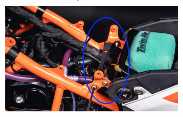
b/ Install the heat shield from ThermoTec on the tank. For easier installation you get the sticker in 2-3 pieces.
