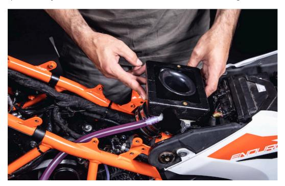
$\mbox{d}/\mbox{ Use the cage and frame to mount the foam filter (ensure it is pre-oiled).}$
