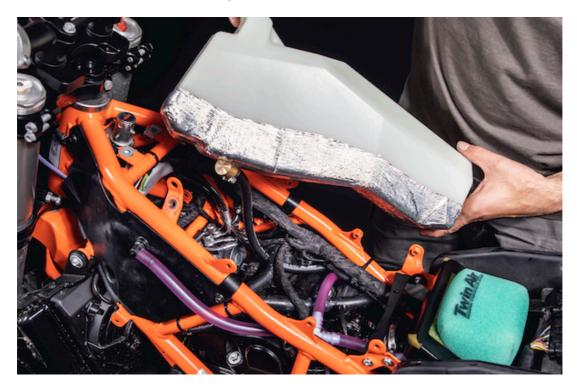
e/To secure the tank, prepare the Velcro strap. Wrap it around the frame, go over the tank, under the frame on the other side and press the tank down to the frame and bracket, secure the Velcro.
