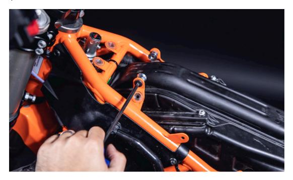
b/ Next remove the four bolts holding the OEM airbox. Note: on the right side the access to the front bolt is hidden under the small radiator. Therefore, you have to remove the radiator first.
