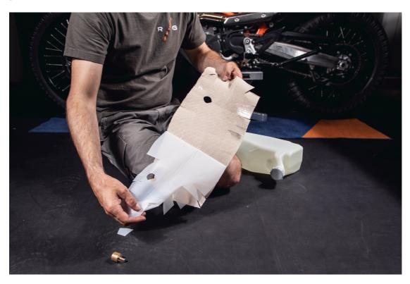
c/ Remove the OEM grommets and use the supplied threat inserts instead.
