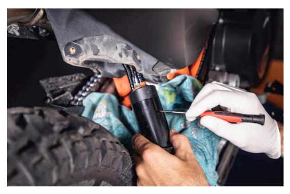
c/ Against the spacer outflow drill a hole diameter 8-10mm. Before you insert the spacer put the fuel tube on the banjo. It is easier to do when removed. But do NOT tight the banjo bolt yet!
